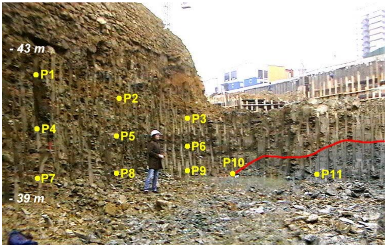
Fig. 3 - Location of samples P1 - P11, collected from site 179 (the red line separates the yellow clays found on the top, from the grey clays).
